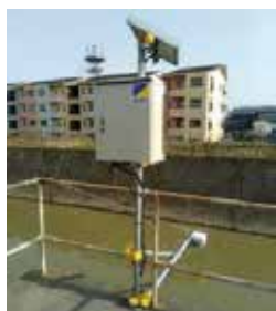
Ultrasonic-type level gauge
